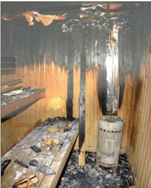
As part of the investigation into the cause of one particular fire, Burgoynes and one of our leading competitors commissioned tests at EXOVA (formerly Warrington Fire Research) on a mock-up of a working sauna cubicle fitted with an exposed heater. The cabin was fitted with thermocouples in order to measure the temperatures achieved under a variety of
